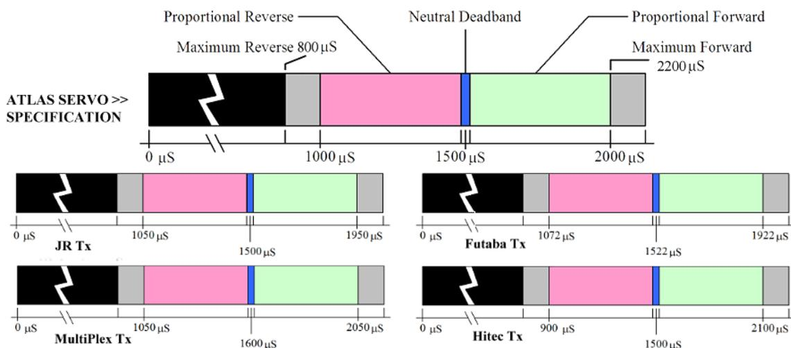
**Gyro Compatibility:** Hyperion ATLAS Digital Servos are able to accept frame rates from 20Hz to 270Hz. As such they are well matched to the majority of Helicopter Gyro systems on the market today and work perfectly with popular Gyros such as Futaba GY401. However, ATLAS servos are NOT compatible certain high-end Gyros which use very short pulse width, such as Futaba GY 611 (870us total pulse). As such, we suggest using only the manufacturer's dedicated servo with such Gyros.
