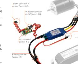
3.1 Maximum Voltage: To determine the maximum number of cells in Series (S) you may use with each controller, divide the rated voltage (for example, 26V) by the Max Charge Voltage for the cell type you use and round down. For example, LiPo at 4.2V/Cell with a 26V ESC: 26/4.2 = 6.19 so 6S LiPo is the maximum
