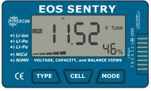
The voltage displayed will not change when you change the pack type, but the estimated capacity will, since the different chemistries have different nominal voltages.
