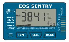
Clicking the MODE button again shows the voltage of the Highest cell and it's number in the top.
