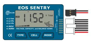
Connecting a pack to the EOS Sentry, NiCd and NiMH packs are connected to the 3 pin connector, LiPo, Lilon and LiFe are connected to the 8 pin connector
