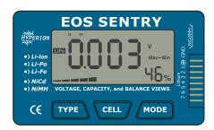
Clicking the MODE button now will bring up the Cell Gap display, showing the voltage difference between the lowest and the highest cells, and shows the cell number of each at the top of the display
