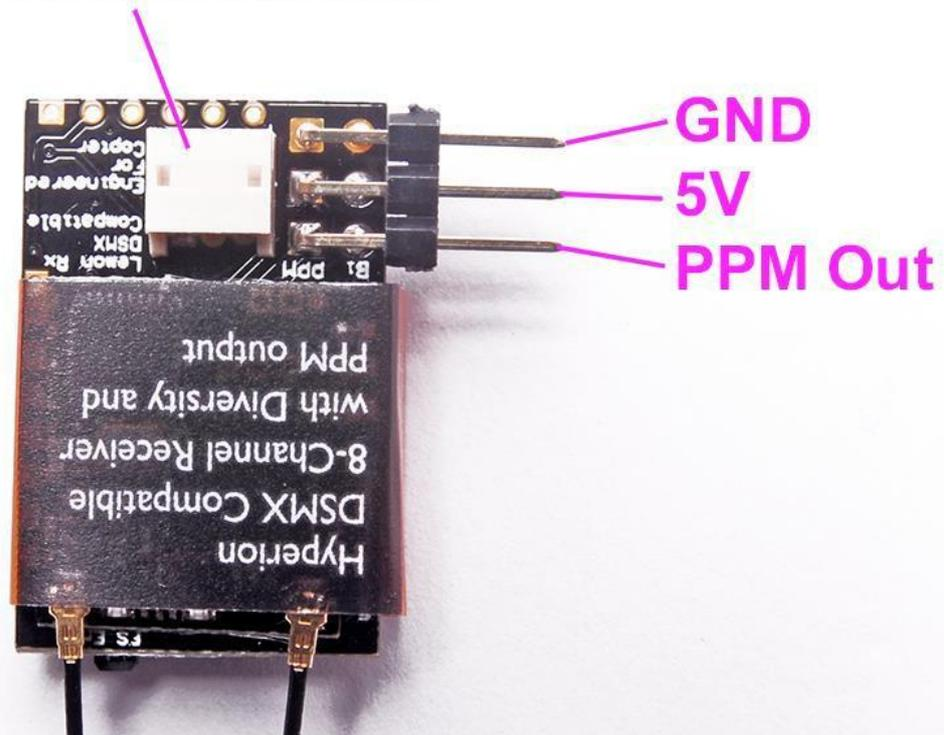
The Hyperion DSMX and DSM2-compatible satellites look similar but the plastic housing is marked with the letters "DSMX" or "DSM2" (obliterated in the photo). The correct satellite should be used with a receiver.
