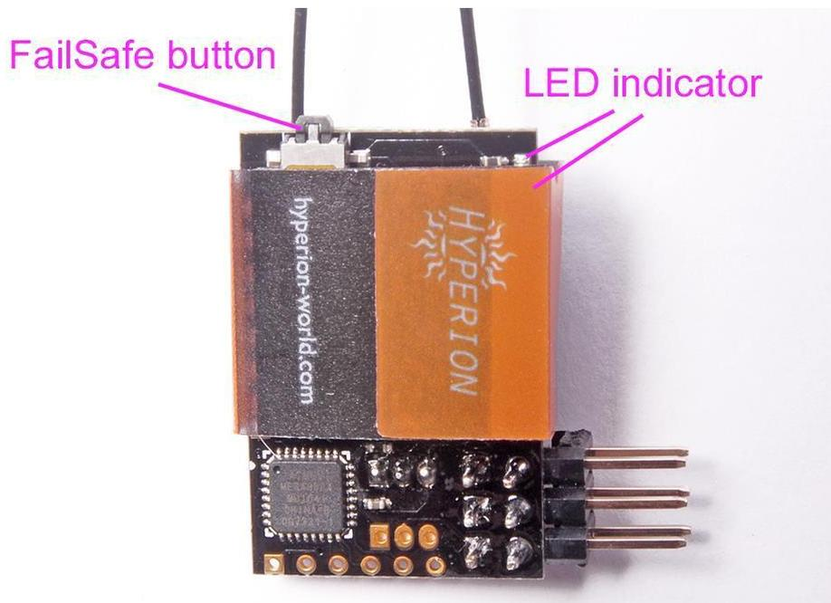
This receiver does not allow for connection of servos or a speed control. It is designed to provide a PPM (also called cPPM) stream suitable for use by a flight controller (or in a wireless trainer system or flight simulator).
